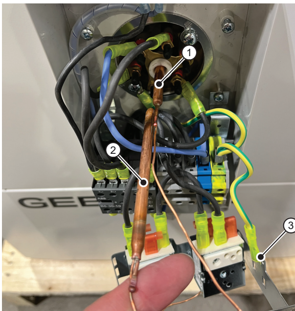
Figure 3.6 - Installing the capillary sensors
